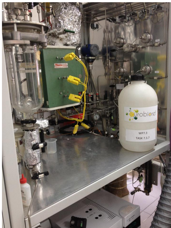
Figure 8. Production of 3.5 kg of higher alcohols from CERTH test unit
